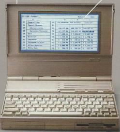
Easily rechargeable, removable internal battery pack gives you hours of use away from a power source
